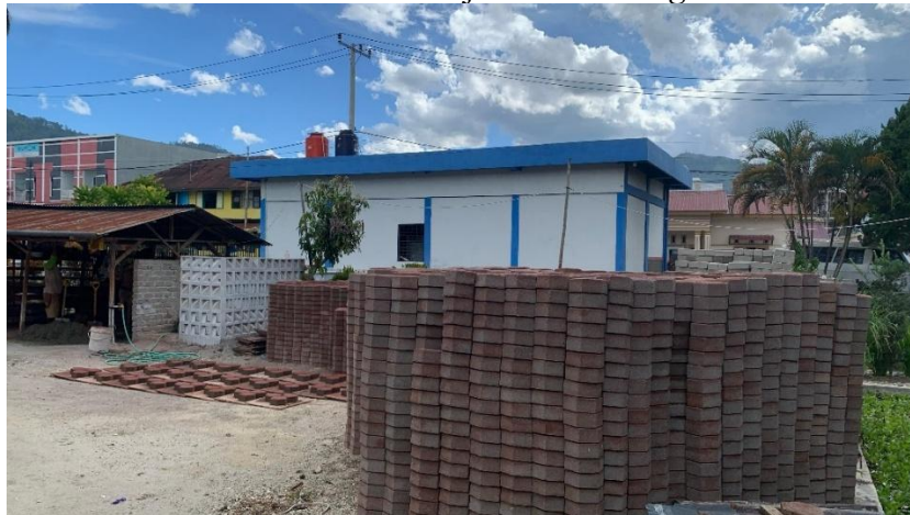
Gambar 1 Proses Penjemuran Pavingblock
